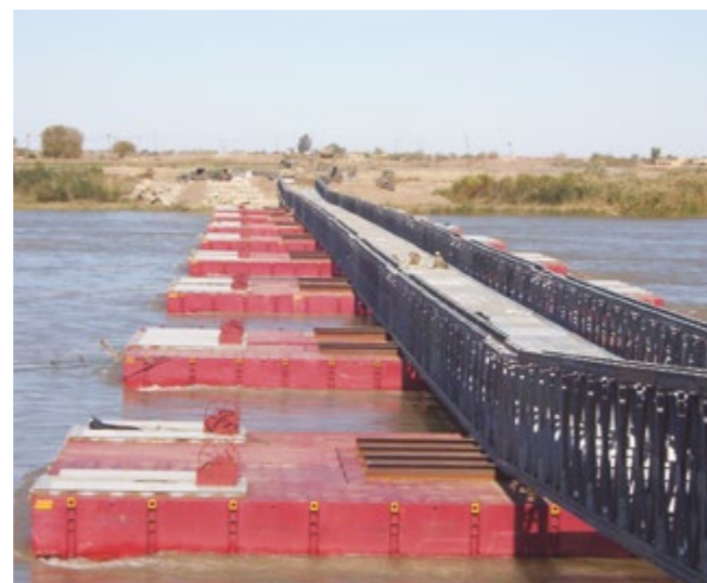
Floating LSB™ with pontoons in Iraq
